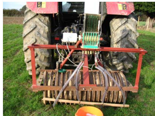
23. Phase 2 – Adapted direct drill (developed by Sandhurst Farm)
